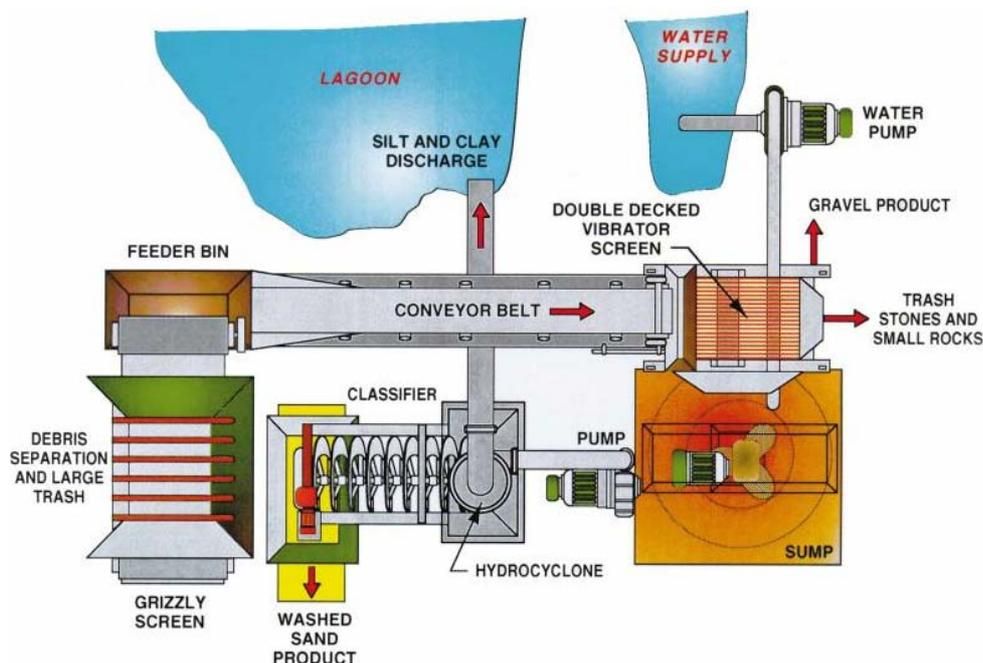
**Figure 10:** Dutch Pilot Plant for separating litter and trash from dredged material
