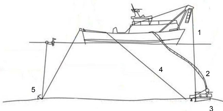
1. Cable to lower and raise the metal cage;
