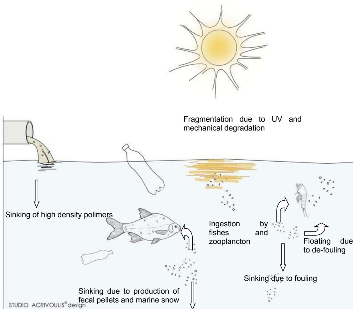
**Figure 3:** Potential pathways for the transport of microplastics on seabed (modified from Wright et al., 2013a)
