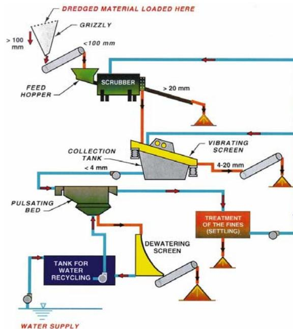
**Figure 9:** Minnesota Pilot Plant for separating litter and trash from dredged material (from Meyers and Adrian, 2000)
