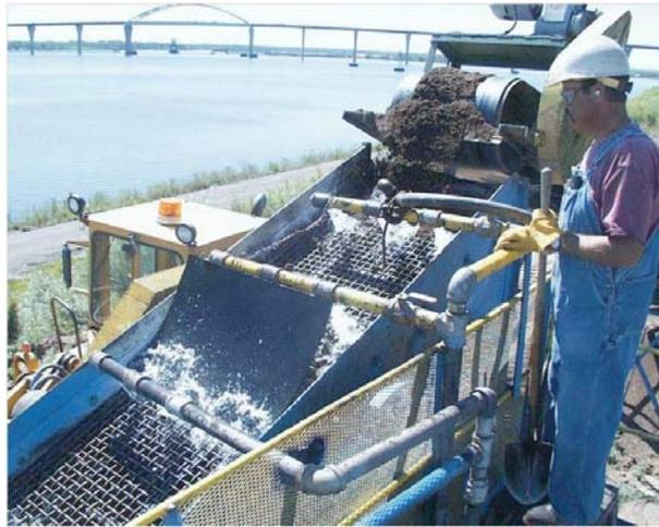
**Figure 8:** Example of vibrating screen (from Spaine et al., 2001)
